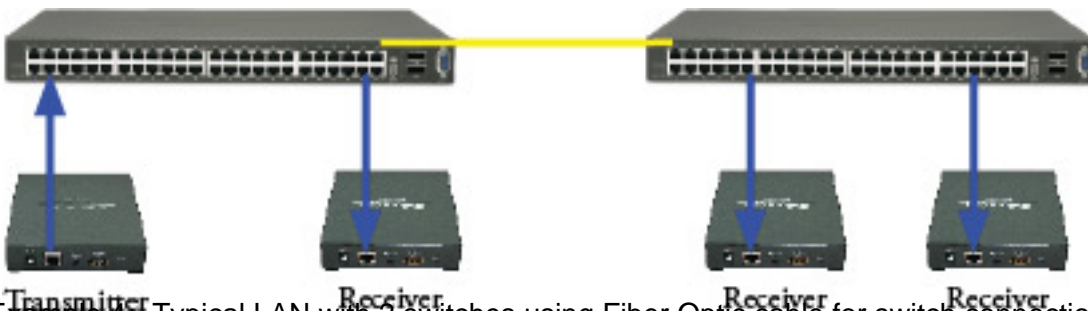
Example 4 - Typical LAN with 2 switches using Fiber Optic cable for switch connection - 2 Layers, 1 Transmitter, and 3 Receivers.
